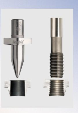
THERMAL FRICTION DRILLING
