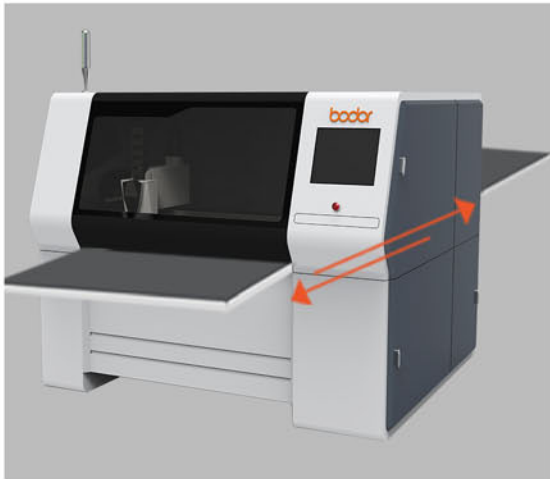
Back open to put the long material through
