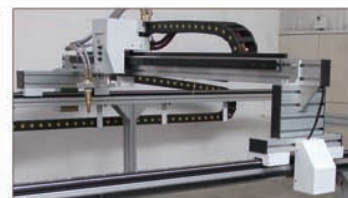
Dual-side precision sliders system, both sides of the crossbeam; increasing the machine stability and to reduces machine vibration. Dual drive system, that can handle more weight.
