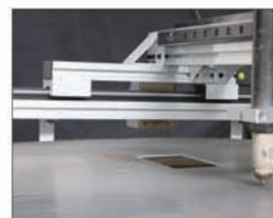
Dual-side precision sliders system, both sides of the crossbeam; increasing the machine stability and to reduces machine vibration. Dual drive system, that can handle more weight.
